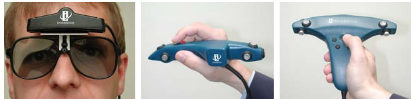
Abb. 5 3D-Sensoren des IS-900-Trackingsystems: Headtracker (an Brille), Stylus, Wand
